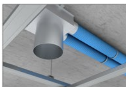
2. Connection to plenum box
